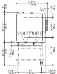
CWII Cold Water inlet 1 CWI2 Cold Water Inlet 2 Electrical inlet (power) Gas connection
